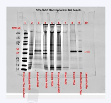
Figure 2: SDS-PAGE electrophoresis gel results for the gel run on Nov. 30, 2020: Precision Plus standard, uninduced PAGE, induced PAGE, insoluble PAGE, soluble PAGE, flow through PAGE, wash PAGE, eluate PAGE, desalted eluate PAGE, and Laemmli buffer. Note the bands near the 43kDa mark as they are indicative of the presence of the GST-DHFR-His protein (Bio-Rad Laboratories, Inc., n.d.). Image from Bio-Rad Laboratories, Inc., n.d., pg. 213.
